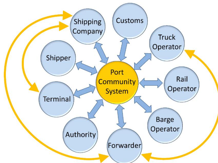
Fig. 1 Multilateral communication network in port traffic with exemplary bilateral communication processes (Meyer-Larsen, 2019)
